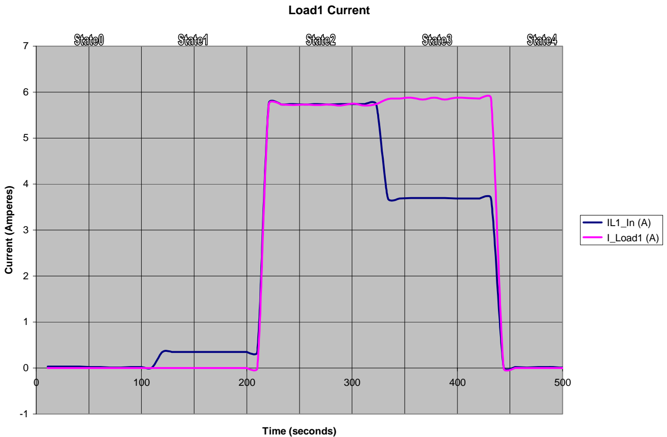
Figure 7 Current for Load 1
